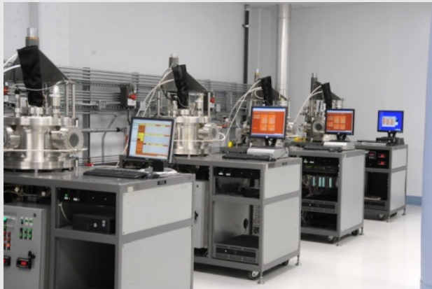
CVD reactors (left) and growth of diamond on seed plates (right) © Scio Diamonds
